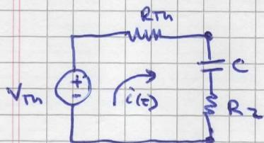
$$V_m = V_{Rm} + V_C + V_{R2}$$
