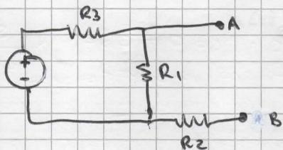
$$R_m = (R_3 // R_1) + R_2 \\ = 7,222 \text{ M}\Omega$$
