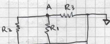
$$R_{th} = \frac{R_1 \times R_3}{R_1 + R_3} = \frac{4M \times 5M}{4M + 5M} = 2,222M\Omega$$
